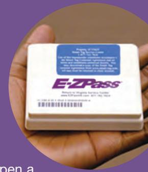
To use E-ZPass, you must first open a prepaid account, and then attach an E-ZPass electronic transponder to your car windshield. Each E-ZPass transponder contains a battery-powered electronic chip with a unique identification code, so when you pass through a toll lane, the toll will be electronically deducted from your account.
